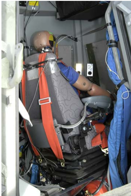
Figure 2: Crash dummy Hybrid III in driver's seat.
