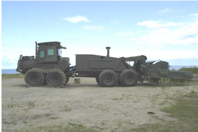
Figure 1: Mine Clearance Vehicle 1 /T deep mine clearance machine
