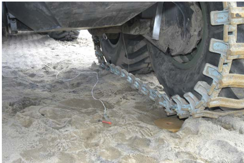
Figure 3: Location of the mine under the right rear wheel.
