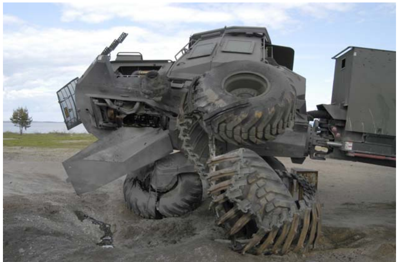
Figure 7: The vehicle viewed from the left with loose engine belly plate.
